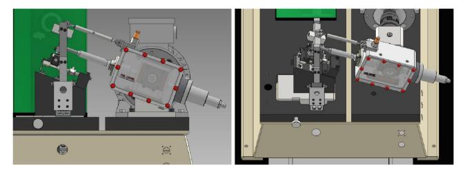
We have designed an adapter that allows tests to be run at short stroke, with the TE 77 reciprocating mechanism rotated through 20 degrees.
