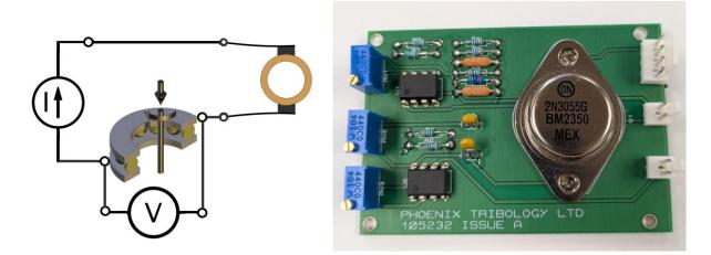
This is a schematic of the LCR Low Resistance Measurement Circuit, which incorporates a constant current source, producing a voltage output proportional to the resistance of the tribocontact. Although schematically a very simple circuit, practical implementation is somewhat more complcated.
