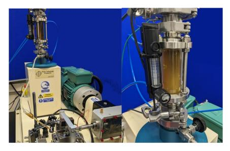
We are running a series of tests on TE 77, using the oil treatment reactor and a marine engine lubricant, which is subjected to exposure to gaseous ammonia and steam. The lubricant is drip fed onto the specimen contact, drains from the specimen bath, and is then pumped back to the top of the reactor. The aim is to see if we can detect any changes in friction and wear response, compared with running air only with treatment. We will be presenting our results at the STLE Annual Meeting.
