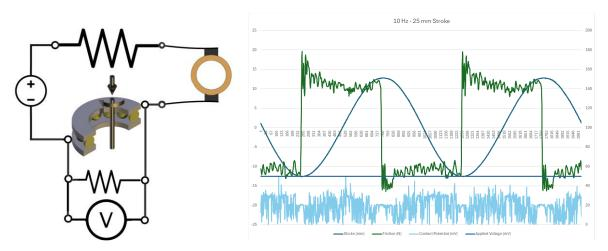
This is the original Lunn-Furey Electrical Contact Resistance Circuit, fitted to numerous different tribometers. It is essentially a high ratio potential divider with the tribo-contact acting as an electrical switch, in parallel with the low resistance side of the potential divider, with the resulting voltage being measured. The voltage across the tribo-contact is typically set to a maximum of between 20 and 50 mV.
