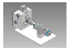
Our new design uses gears to set the slide-roll ratio, much as in the <u>**TE 53 Multi-Purpose</u>** <u>**Friction & Wear Tester**</u>. The maximum specimen speed, with contact slip, is 6,000 rpm. At zero slide-roll ratio, with the gears removed, the maximum specimen speed is 12,000 rpm. The two lower rollers are electrically insulated for ECR measurement and the traction between the upper roller and the specimen roller is measured with a force transducer.</u>
