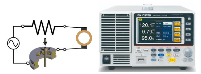
This is the Programmable Continuous AC/DC Current Source Circuit. It allows a current of up to 1 amp to be passed through the tribo-contact. This is the sort of continuous current that might be generated in large rotating electrical machinery.
