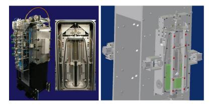
The original TE 104 machine is designed to run under pressurised hydrogen, which adds considerably to the cost and complexity of the machine. We have a client who wants a similar device, but without the hydrogen capability, for running tests in non-explosive gases. We can achieve what is required by removing the outer nitrogen chamber and all the hydrogen and explosion rated components from the original TE 104. This means we will end up with two machines that we will designate as:
