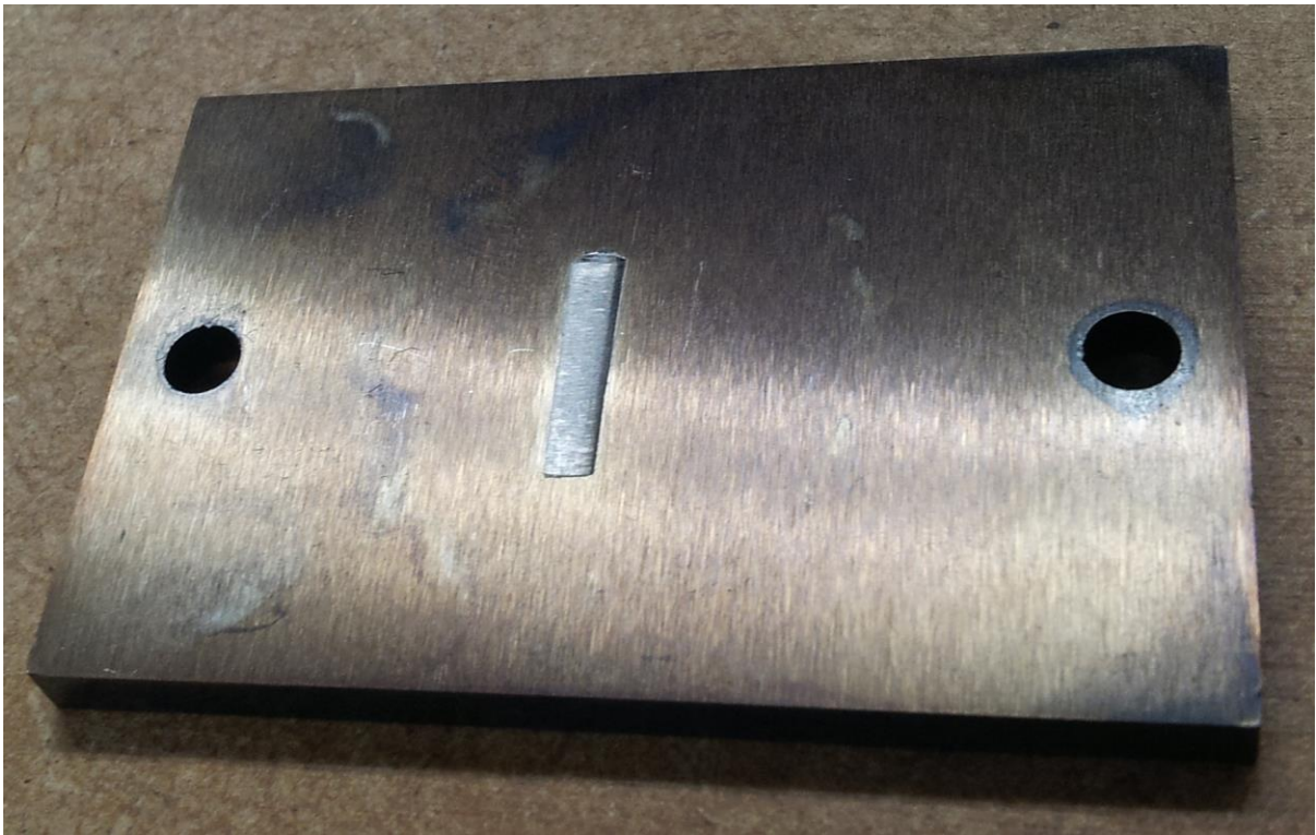
Figure 7: Test Sample – Wear Scar Depth ~ 90 microns
