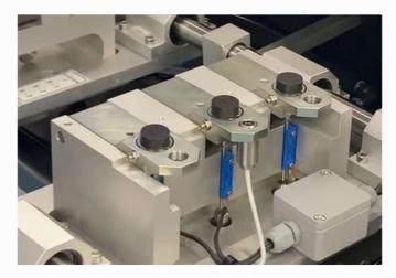
The four pin carrier assemblies are mounted on linear bearing rails, with each carrier restrained from movement by a strain gauge force transducer, which senses the total friction force generated by each set of three pins.
