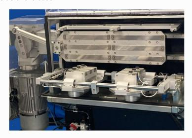
Pin specimens are mounted in lever arms with pivot points perpendicular to the sliding direction. Pin lever assemblies are mounted in groups of three, on separate tracks, to allow each pin to run against its own specimen plate.
