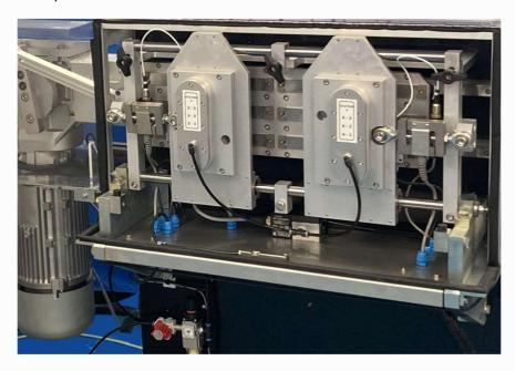
Load is applied to each pin using a pin cylinder, with air pressure applied through common manifolds and set by a precision manual pressure regulator. A pressure transducer is provided, calibrated to display the corresponding load. At 8 bar applied pressure each pin cylinder generates a force of 133 N.
